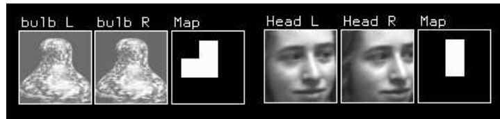
Figure 3: Left: A synthetic stereo pair, showing a textured pear-shaped object, and the output of a hyperbolic patch detector (white = hyperbolic). The pear’s neck has been correctly classified as most likely to be hyperbolic. Right: The same operator applied to two frames of a motion sequence of a rotating human head. The bridge of the nose has been correctly classified as hyperbolic.
